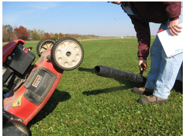
Fig. 4. The deck of the mower was cleaned with a blower to remove debris and reduce the potential to track herbicide from one plot to another.
