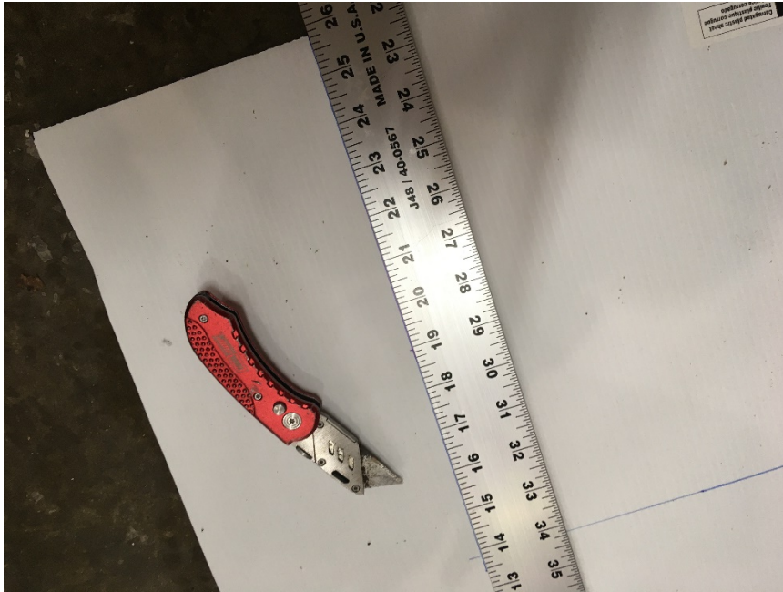
Figure 7. Use a ruler to guide your cutting with a razor blade.
