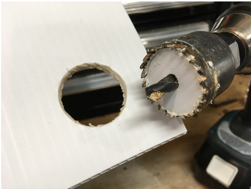
Figure 12. Carefully drill out each corner marked. Place a scrap piece of wood below the cut to keep from bending the platform and to help provide a cleaner cut.
