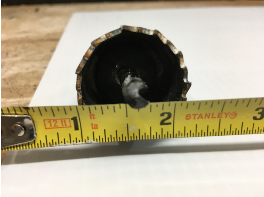
Figure 11. Use a hole saw drill bit 1.125 or 1.25 inches in diameter.
